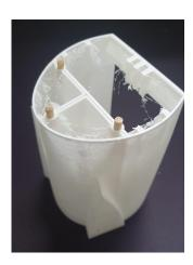
Glue sections 1,2,3 and 4 of the fuse and together.
