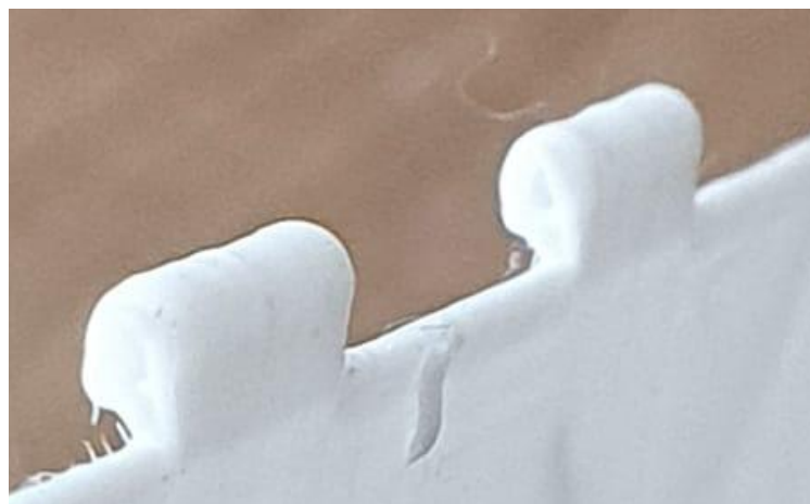
Faulty first layers of hinge
