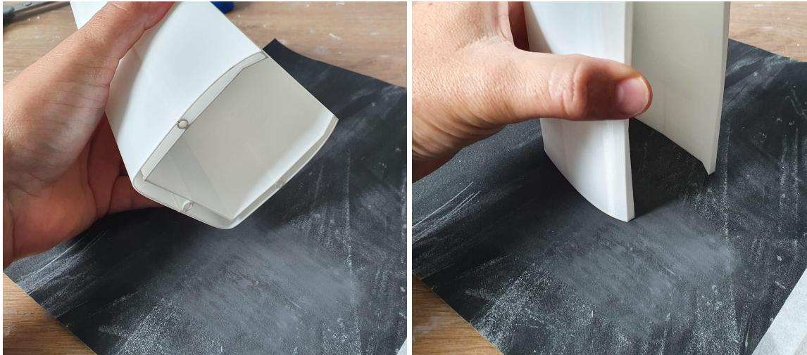
Almost all components which are to be joined will have 3mm alignment pin holes printed into the mating faces of the parts. Cut 10mm sections of 3mm skewer and place them into the alignment holes.
