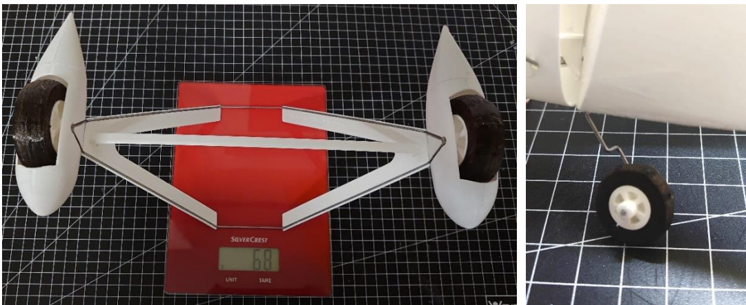
Figure 9: Weight-optimized landing gear and tail wheel
