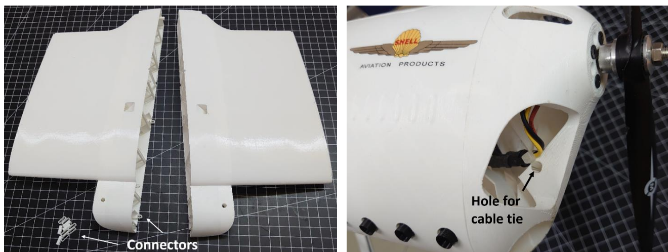
Figure 10: Connectors are available to simplify the alignment of left- and right-wing halves (left). Motor cables can be fixed to the fuselage (right).
