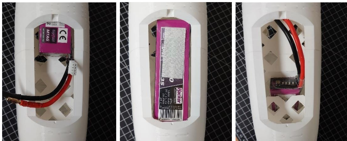
Figure 11: Extended battery compartment to adjust center of gravity.
