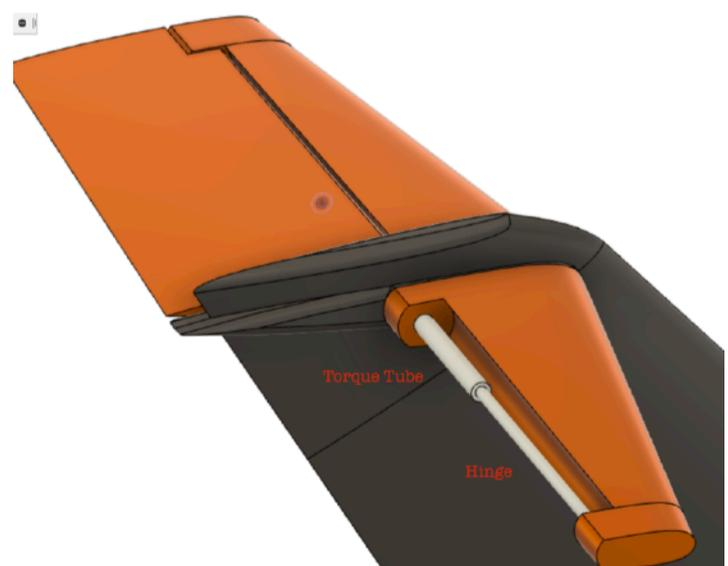
surface of the elevator. The control rod needs to be made of piano wire that is flexible enough to bend a little through the curve in the Bowden.
