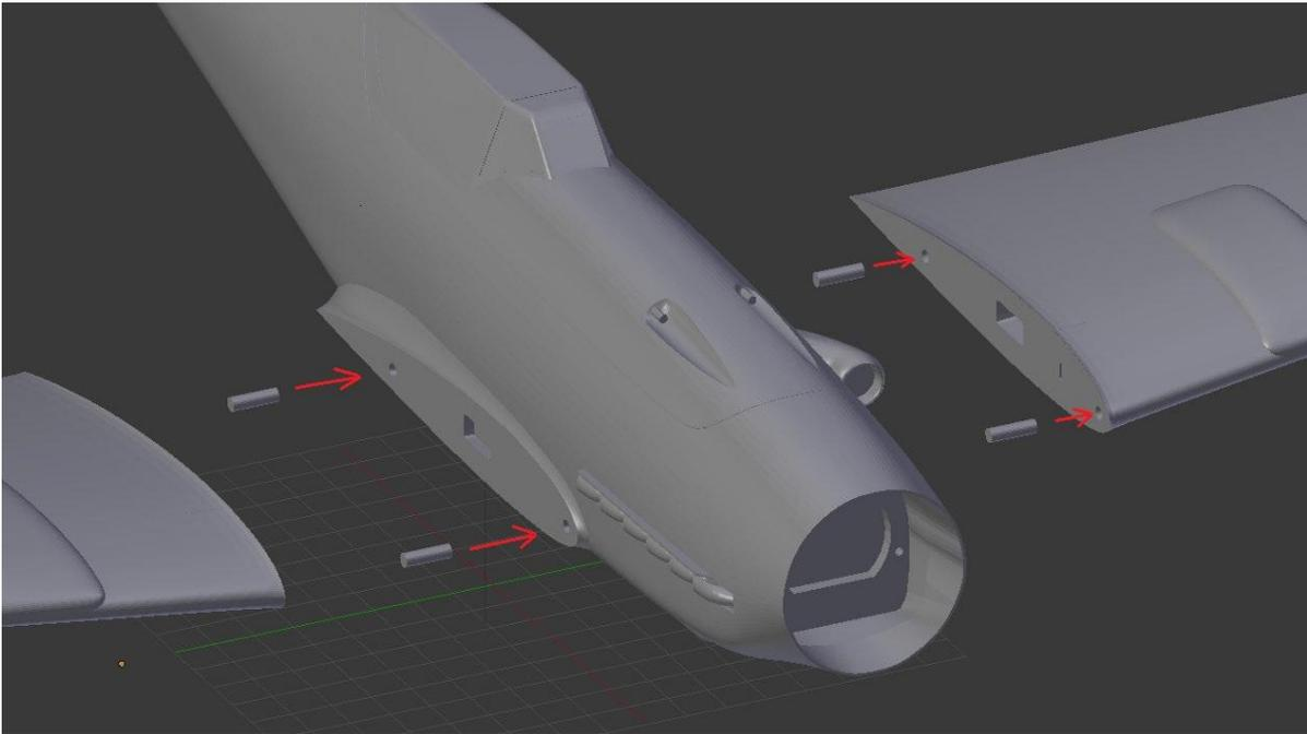
Glue the wings to the fuselage **NOTE** – if using 3mm x 0.6mm carbon strip, now is the time to install it. Simply slide the carbon strip into the slot and cut it so it does not protrude out of the wing (circled in red, see image). The cross structure of the fuselage spreads the load of the wings at the root which negates the need of a connecting spar in the fuselage.
