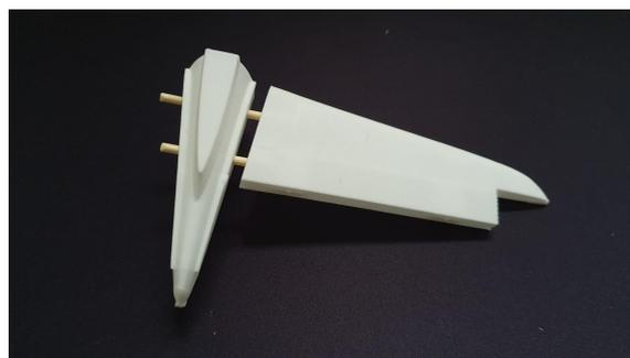
Bend a section of 1mm steel wire to connect the elevators together. .
