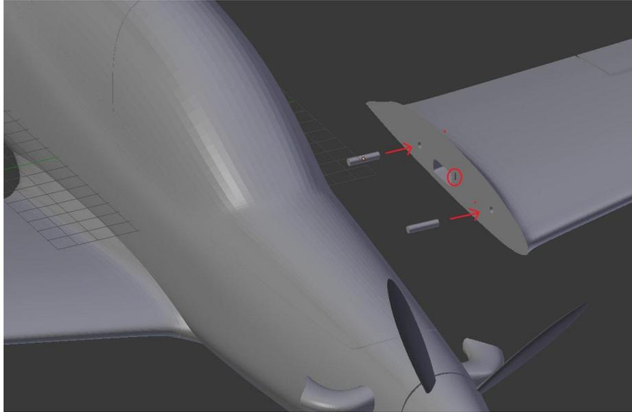
Glue the wings to the fuselage **NOTE** – if using 3mm x 0.6mm carbon strip, now is the time to install it. Simply slide the carbon strip into the slot and cut it so it does not protrude out of the wing (circled in red, see image). The cross structure of the fuselage spreads the load of the wings at the root which negates the need of a connecting spar in the fuselage.
