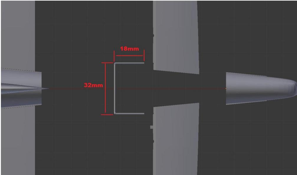
Test fit the wire and the elevators connection to the horizontal stabilisers before gluing the wire to the elevators, or the elevators to the tail plane. There should be un-obstructed travel.
