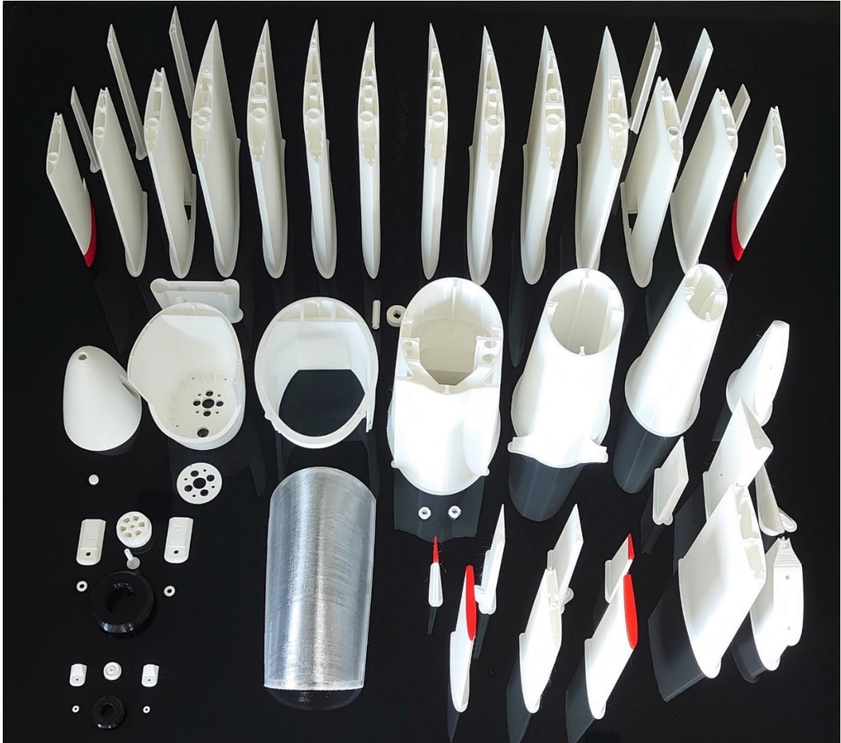
Figure 4: Fresh from the printer - main print parts including wheels (engine version 1.0)
