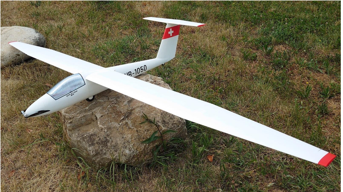
Figure 1: 3D-printed Pilatus B4 with electric engine
