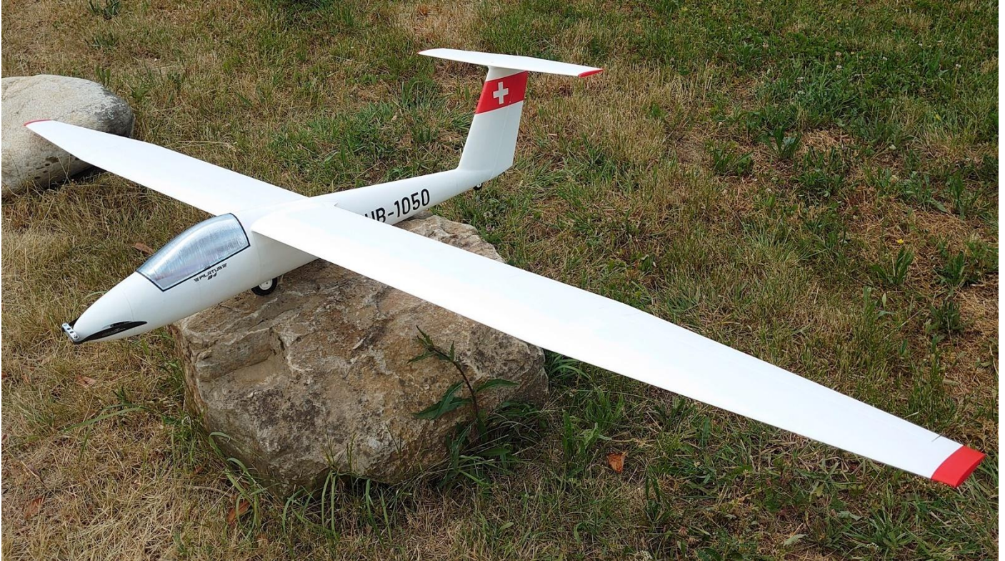
Figure 1: 3D-printed Pilatus B4 with electric engine
