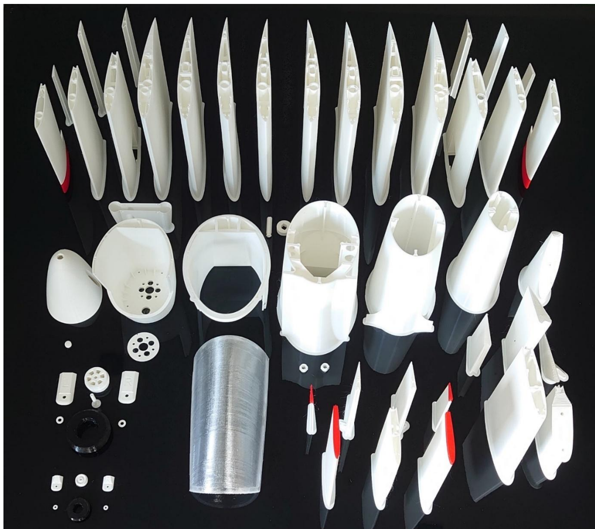
Figure 4: Fresh from the printer - main print parts including wheels (engine version)
